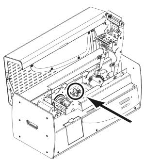
The contact station is a module fitted in the factory. It is located over the path taken by the cards and before the print head. To make contact with the station, the smartcard is positioned underneath it and is pushed mechanically upwards. The programming sequence for a smartcard is always carried out before the printing.
