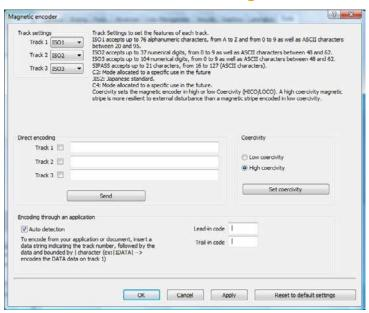
The **Magnetic Encoder** dialog box opens when the **Encoding Settings** button is selected.
