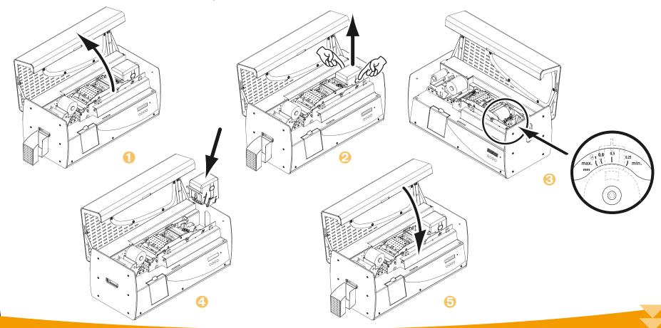
Adjusting card thickness from inside of the printer:
