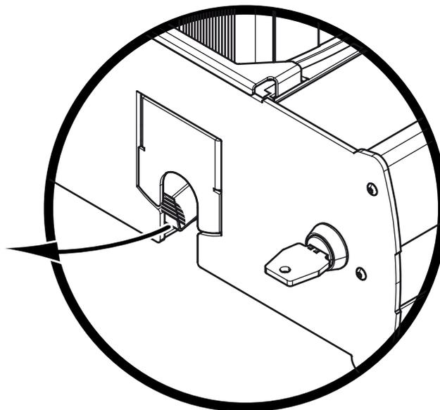
Evolis advises you to empty the reject hopper regularly, such as whenever the ribbon is changed or during routine maintenance. For the standard version (without central locking), it is sufficient just to remove the cards present in the reject hopper.
