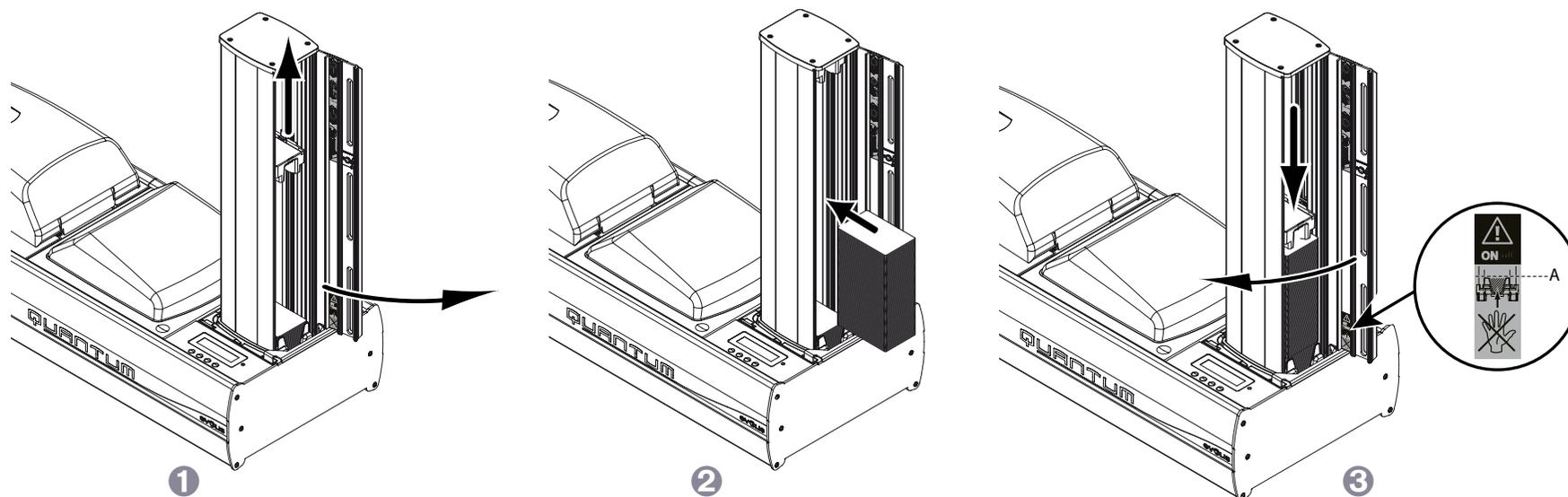
Similarly, it is possible to remove the personalised cards from the output stack in place in the printer when this is executing a job.
