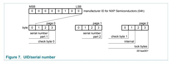
In accordance with ISO/IEC 14443-3 check byte 0 (BCC0) is defined as CT Å SN0 Å SN1 Å SN2. Check byte 1 (BCC1) is defined as SN3 Å SN4 Å SN5 Å SN6.
