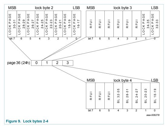
The default value of lock bytes 2-4 is 00 00 00h. The value of byte 3 on page 36 (see Figure 9) is always BDh when read.
