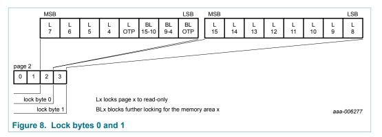
For example if BL15-10 is set to logic 1, then bits L15 to L10 (lock byte 1, bit[7:2]) can no longer be changed. A WRITE command or COMPATIBILITY\_WRITE command to page 02h, sets the locking and block-locking bits. Byte 2 and byte 3 of the WRITE or COMPATIBILITY\_WRITE command, and the contents of the lock bytes are bit-wise OR'ed and the result then becomes the new content of the lock bytes. This process is irreversible. If a bit is set to logic 1, it cannot be changed back to logic 0.
