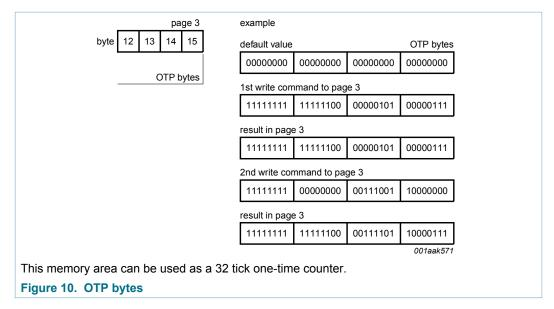
The parameter bytes of the WRITE command and the current contents of the OTP bytes are bit-wise OR'ed. The result is the new OTP byte contents. This process is irreversible and once a bit is set to logic 1, it cannot be changed back to logic 0.
