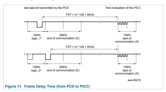
**Remark:** Due to the coding of commands, the measured timings usually excludes (a part of) the end of communication. Consider this factor when comparing the specified times with the measured times.
